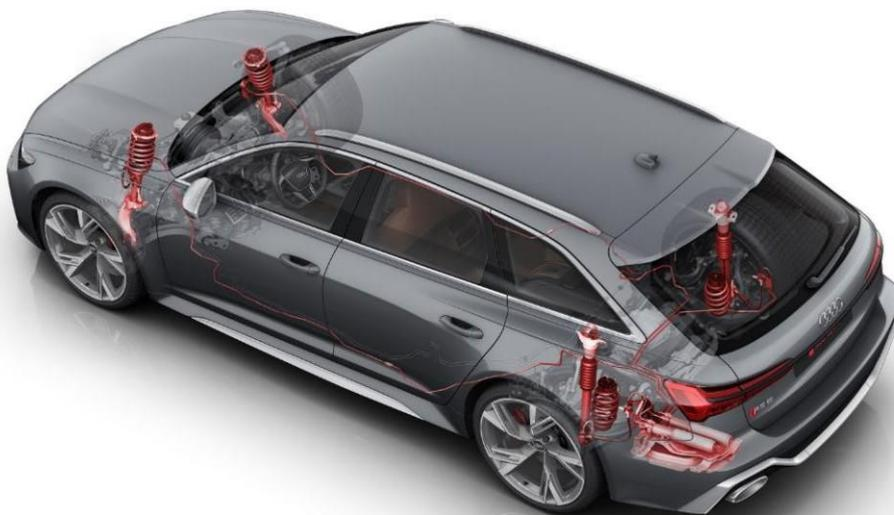
The generation of dampers with integrated valve has a more compact, lighter design and reduces pitch and rolling movements even more effectively. In addition, it enables the damping forces to be spread even more widely between the comfort, auto, and dynamic modes as well as more precise suspension adjustment for high damping forces, which occur during cornering at speed.
